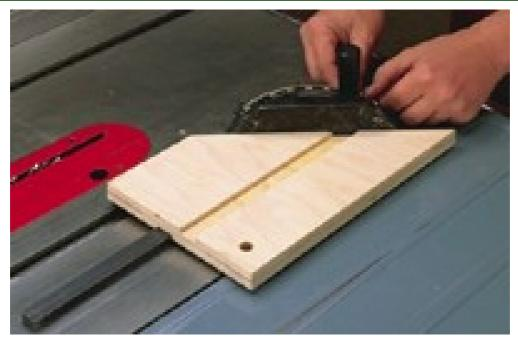
I used to spend quite a bit of time adjusting my mitre gauge and testing the set-up. Now I have a simple jig that allows me to quickly and accurately set the mitre gauge to both 90° and C, see photo.
